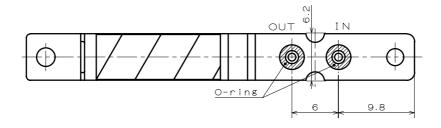
3-valve manifold clamped by screws
